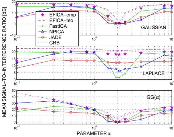
Fig. 1(a) Average SIRs of the three kinds of signals in Example 1.
