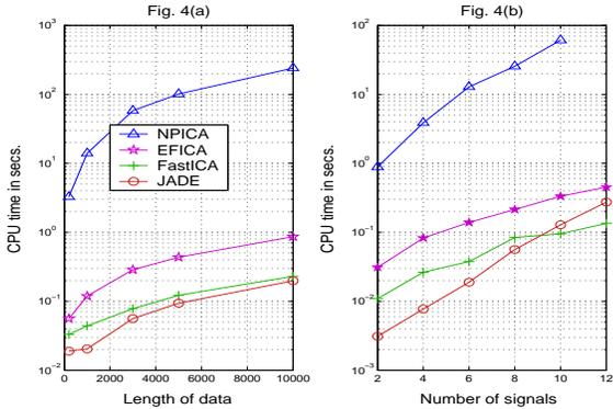
Fig. 4 CPU time needed to separate (a) 6 signals of a various length (b) various # of signals of a fixed length  $N = 1000$ .
