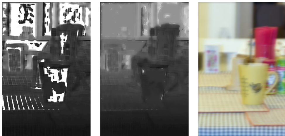
Figure 1: Rough estimation of the depth map (the left image); depth of objects in the scene (the middle image); the final result, estimation of the retinal image (the right image).
