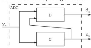
Figure: Internal structure of active fault detector and controller
