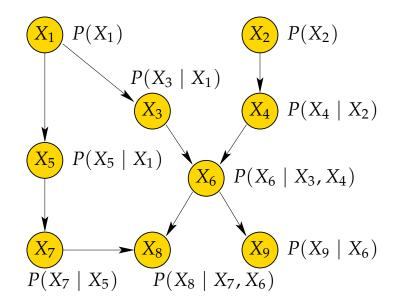
$P(X_{1},...,X_{9}) =$  $= P(X_{9}|X_{8},...,X_{1}) \cdot P(X_{8}|X_{7},...,X_{1}) \cdot ... \cdot P(X_{2}|X_{1}) \cdot P(X_{1})$  $= P(X_{9}|X_{6}) \cdot P(X_{8}|X_{7},X_{6}) \cdot P(X_{7}|X_{5}) \cdot P(X_{6}|X_{4},X_{3})$  $\cdot P(X_{5}|X_{1}) \cdot P(X_{4}|X_{2}) \cdot P(X_{3}|X_{1}) \cdot P(X_{2}) \cdot P(X_{1})$
