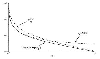
Fig. 2: Asymptotic performance of one unit and symmetric FastICA and the CRB versus parameter  $\kappa$ .
