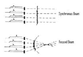
Figure 11: Focusing of Ultrasound Transducer
