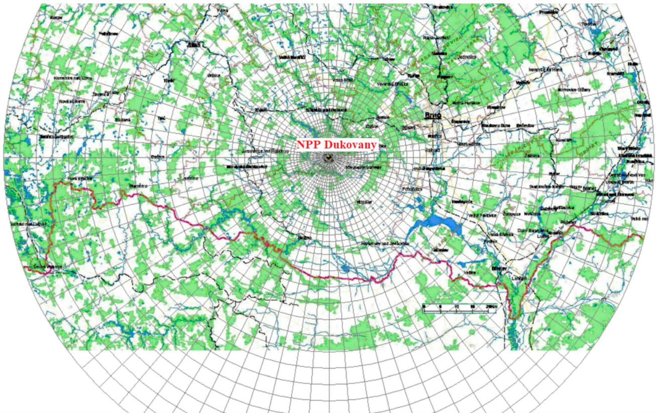
Fig. 1 Polar computational grid on the map background in a vicinity of the Dukovany nuclear power plant. It consists of 42 concentric circles up to 100 kms from the source of pollution and 80 angular beams (clockwise, from North)
